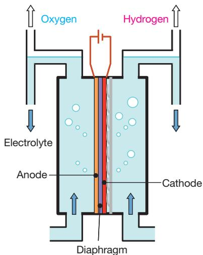
**Fig. 7 Schematic diagram of alkaline water electrolysis cell**
