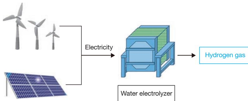
Fig. 2 Process of producing hydrogen by water electrolysis
