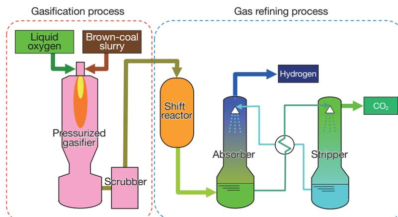
Fig. 3 Process of producing hydrogen by brown-coal gasification
