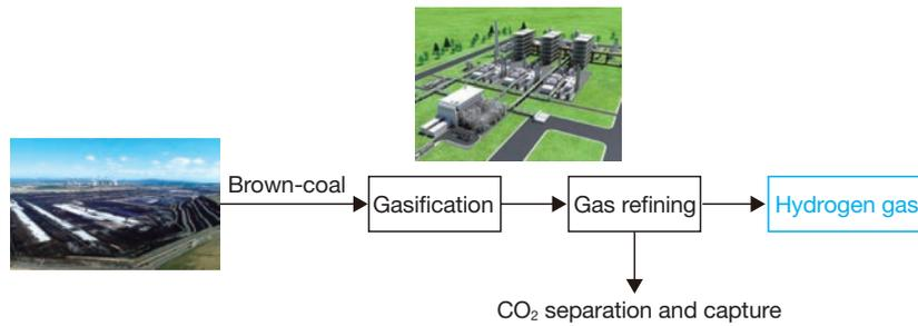
Fig. 1 Process of producing hydrogen from brown-coal
