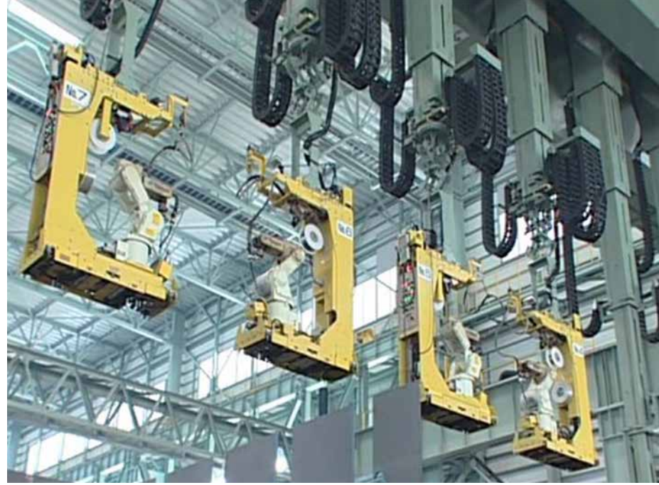
Robots used for welding thick steel plates on ships at Kawasaki's Sakaide Works are good examples of technological advancements propelled by internal needs.
