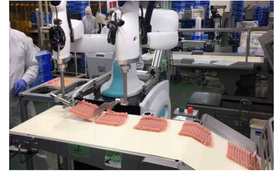
A duAro in the backroom of a supermarket's meat section, transferring cut meat to trays. Using spatulas in both “hands,” meat is packed neatly without being crushed.
