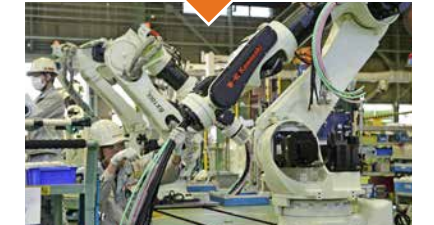
Components of the arm are added, beginning with the lowest section and, at the same time, the motor in the "joint" section of the arm is wired.
