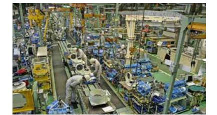
The first step in manufacturing a robot is to assemble a decelerator and an arm base which form the foundation. The arm is then attached to the "black hole."
