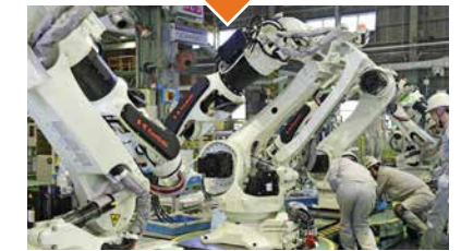
This is an extra-large, general-purpose robot with a payload capacity of 1,500 kg. Optional parts as needed for specific applications are attached to the tip of the arm.
