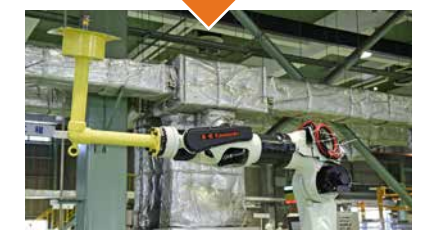
An inspection line for the finished robot: The L-shaped, yellow object is a weight used for inspection. Using this weight, each arm's range of motion, forward/backward, and up/down movements are checked.
