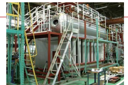
A waste heat boiler for a co-generation system — the fruit of synergy between KHI and KTE
