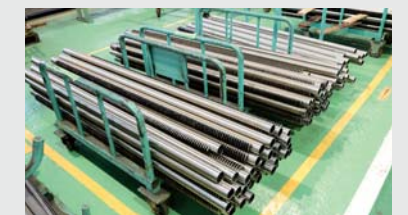
For the once-through boiler's casing, tubes and steel plates (fins) are used. This compact boiler with a steam output of 2,000 kg/h requires 51 tubes.
