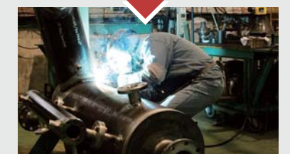
For the once-through boiler's casing, tubes and steel plates (fins) are used. This compact boiler with a steam output of 2,000 kg/h requires 51 tubes.
