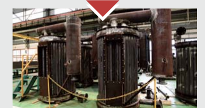
After welding leak tests are conducted, the entire boiler goes through an annealing process to eliminate residual stress, so as to make it capable of withstanding high pressure and achieve prolonged product life.
