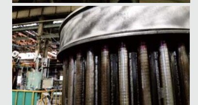
Welding is the key to constructing effective boilers. Tubes and fins are welded to produce the boiler's cylindrical body. At KTE's manufacturing plant, welding robots are widely used for this process.
