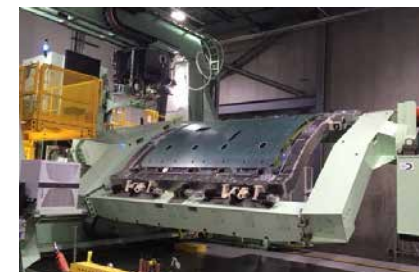
Manufacturing a cargo door using an auto riveter.
