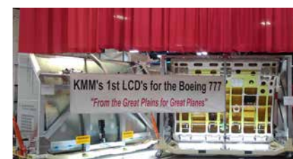
First completed cargo doors.
