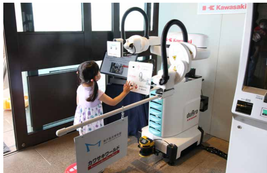
The automatic temperature measurement system installed at Kobe Maritime Museum/Kawasaki Good Times World.
