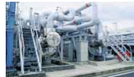
A vaporizer for regasifying LNG by heat exchange.
